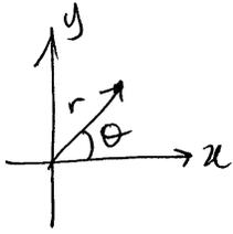
$$\text{donde } \begin{aligned} x &= r \cos \theta & \dot{x} &= \dot{r} \cos \theta - \dot{\theta} r \sin \theta \\ y &= r \sin \theta & \dot{y} &= \dot{r} \sin \theta + \dot{\theta} r \cos \theta \end{aligned}$$
